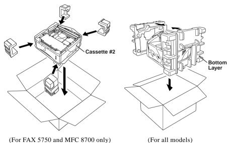
Place documents (manual and printed material) and the drum unit and toner cartridge assembly into the original carton as shown below:
